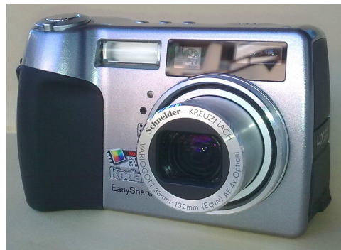
Kodak EasyShare Z 730 digital camera, with range-finder and a sensor of five megapixels (2005).
