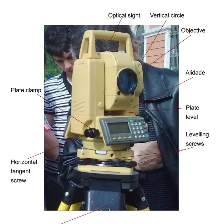
Tripod, to which the theodolite is connected by the centering screw
