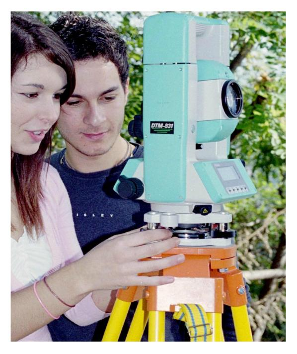
Two levelling screws are rotated *thumbs-in or thumbs-out* to center the plate level vial bubble of Nikon DTM-831 total station, whose sensitivity is 30"/ 2 mm. Its telescope has a magnification of 33 X.
